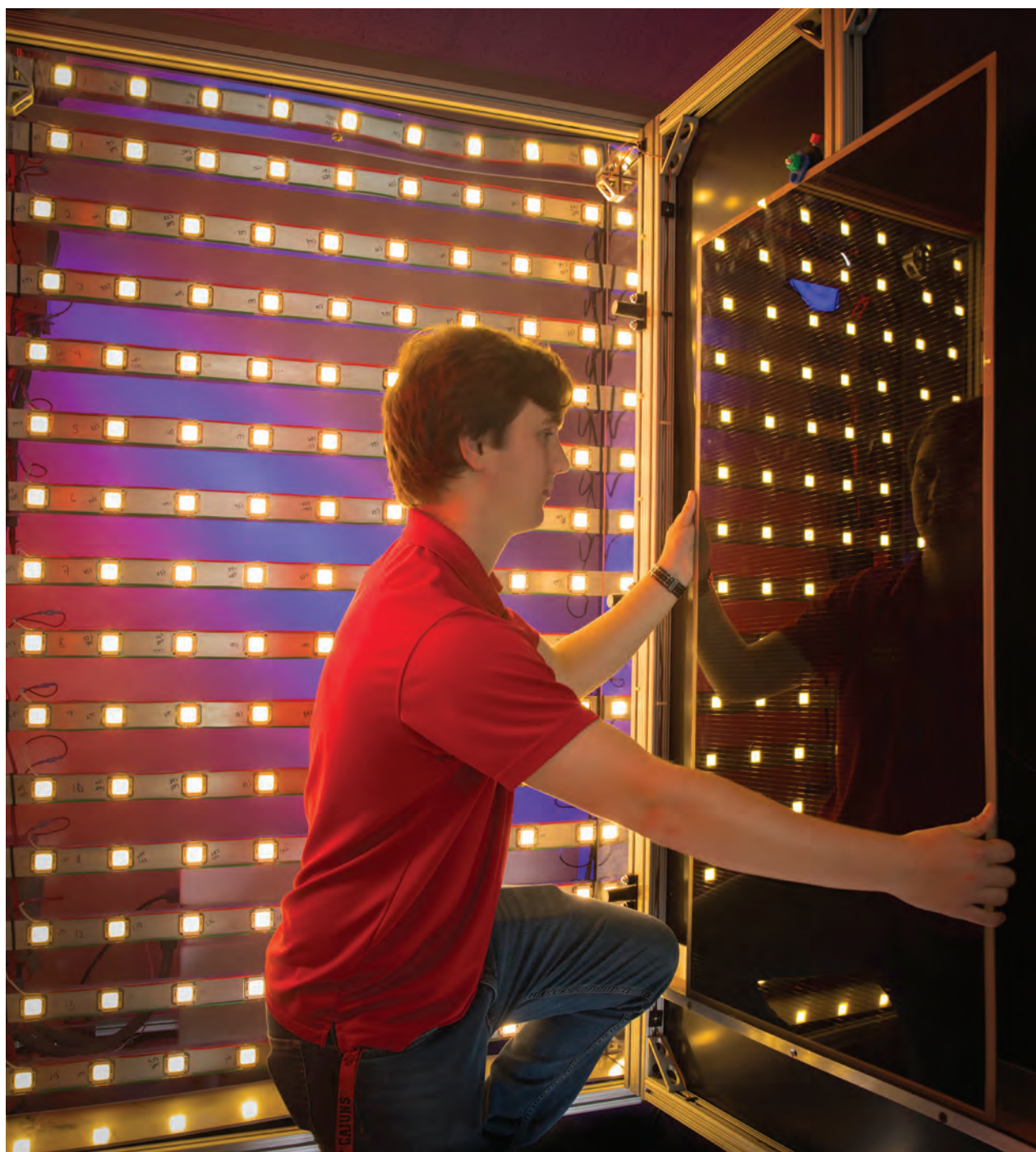
Student Cy Kipp adjusts a solar panel inside the PART Lab's flash tester, or artificial sun.
