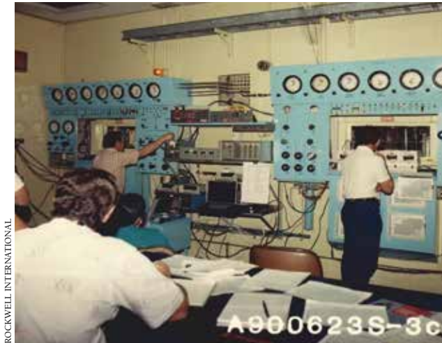
Team engineers view testing of liquid hydrogen behind bulletproof glass in an explosion-proof control room.
