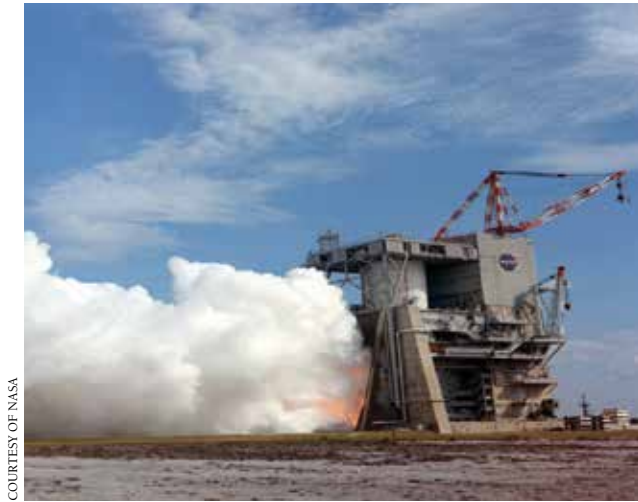
Test-firing of the S-II stage of the Saturn V rocket was conducted at a facility in Mississippi.
